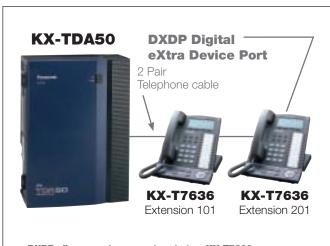
DXDP allows you to connect up to two KX-T7600 Digital Telephones to the same system port, each can be assigned a different telephone number and operate independently at the same time.
